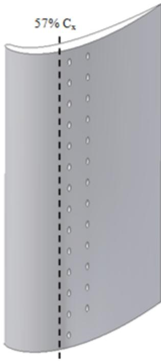
**Fig 2** L1A blade section with approximate location of separation line in steady flow.
