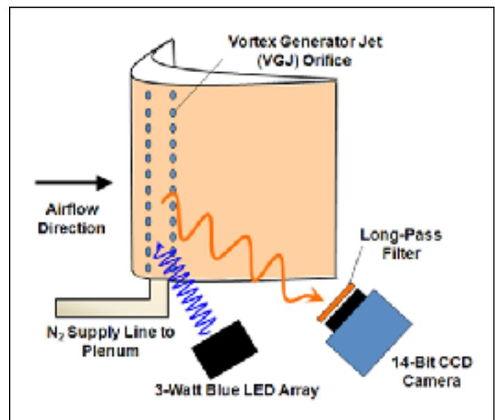
**Fig 3** Experimental setup showing L1A turbine blade painted with PC-PSP (acrylic duct walls and second L1A blade not shown).
