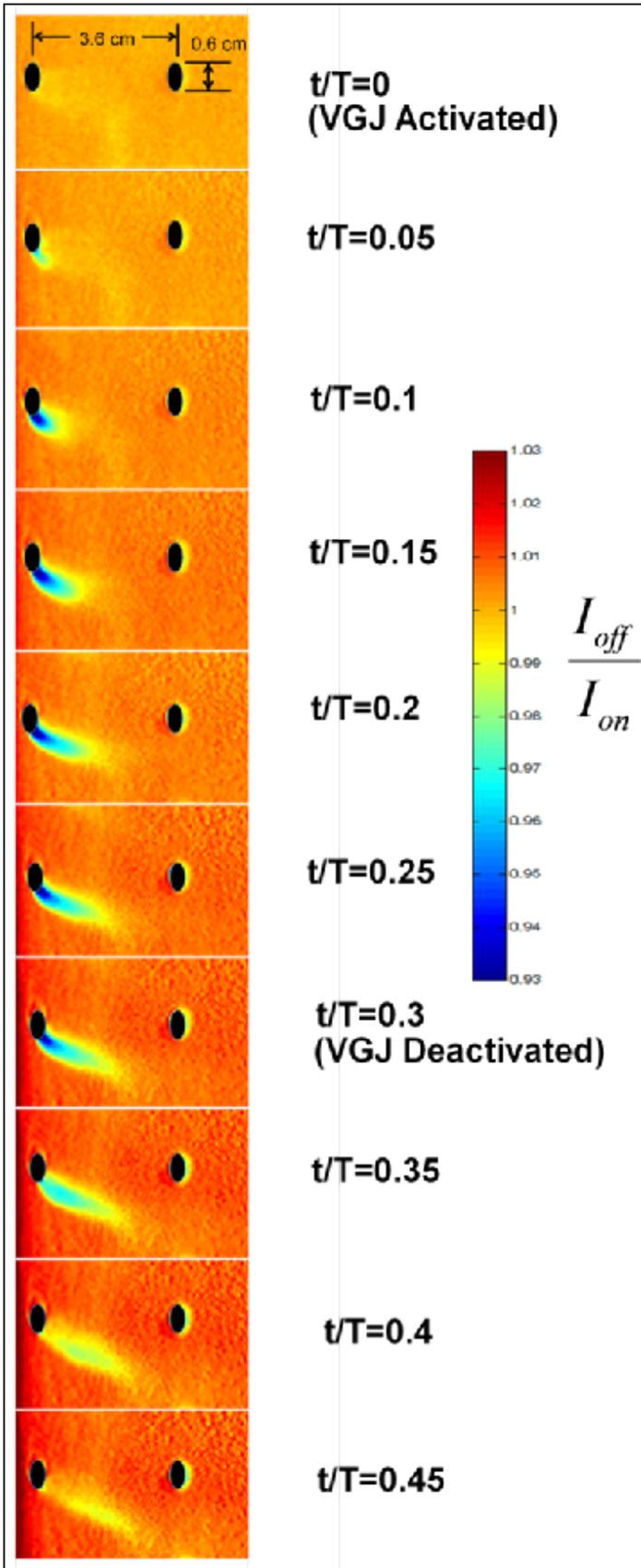
**Fig 4** Time-resolved image sequence of single VGJ for  $t/T=0$  to 35% of pulsing period.
