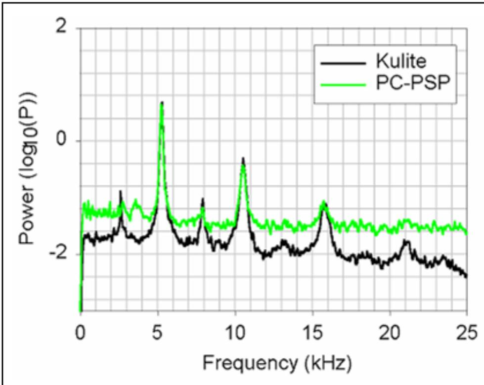
**Fig 1** Frequency response characteristics for PC-PSP and a Kulite™ pressure transducer at a point in the fluidic oscillator flow field. (From Gregory [4]).
