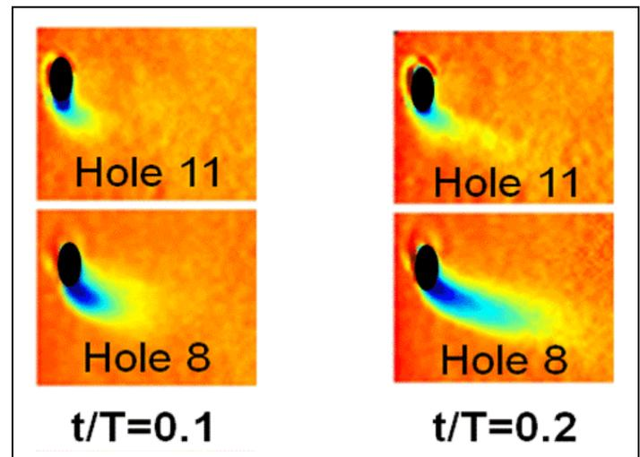
Fig 5 Nonuniformity between two holes on upstream VGJ row.
