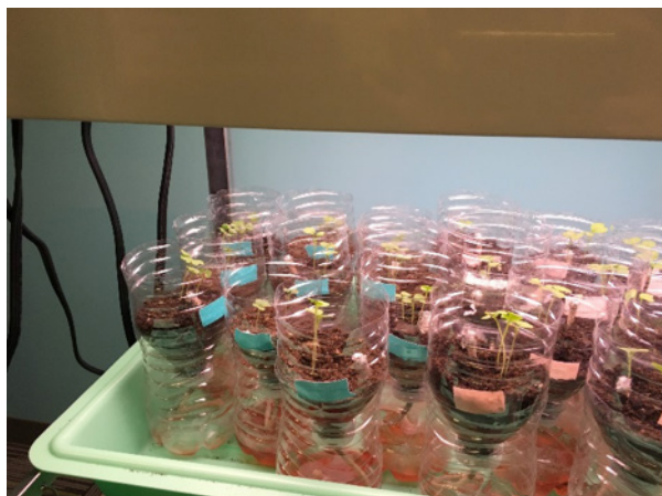
Figure 1. The watering pots and watering wick system. The colored labels indicate a specific solution (blue=0.5% PQQ solution, pink=0.25% PQQ solution).
